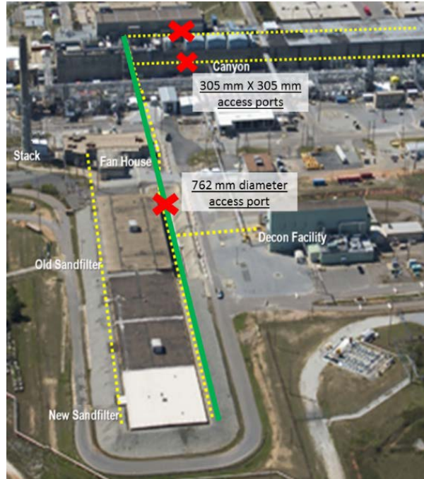
Fig. 2: Approximate location of tunnels (green and yellow dashed) and access points.
