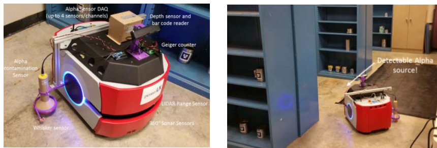
Fig. 7: (Left) Modified Pioneer LX with Geiger counter, alpha sensor, & object recognition. (Right) UT Austin's mock storage vault.
