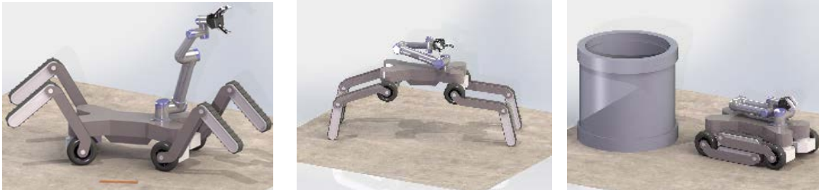
Fig. 12: The proposed multi-purpose crawler for comprehensive inspection of the CAEX tunnel. The platform can move via wheels, tracks or legged locomotion.
